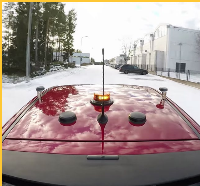
..... Marilyn 2.0, a Citroen C4 retrofitted with AV technology, cruises around the snowy streets of Tampere's UrbanAutoTest. (Credit: VTT)
