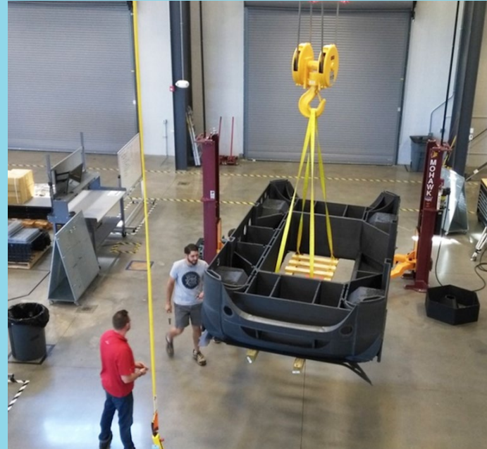
..... In 2014, Local Motors microfactory based in Knoxville partnered with the Department of Energy's Oak Ridge National Laboratory to produce the world's first 3-D printed car. (Credit: Local Motors)
