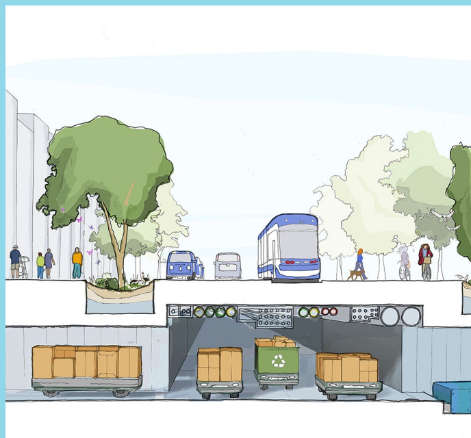
A proposed design for the redevelopment of Toronto's Quayside waterfront district by Sidewalk Labs, part of Google's Alphabet family, will feature a subterranean network of AV freight conveyors. (Credit: Sidewalk Labs)
